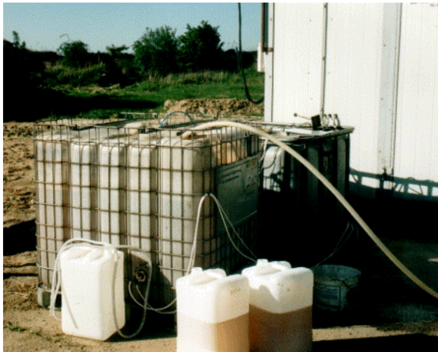
Fig. 1.14. Bioreactors with aeration and temperature control systems
