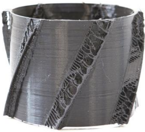
Fig. 4. 6 ribs with 30°, extrusion 5 mm, V_{rib} : 400mm/min, V_{cyl} : 800 mm/min
