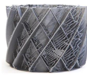
Fig. 9. 12 ribs with 60° and - 60°, extrusion 5 mm, V_{rib} : 400 mm/min, V_{cyl} : 800 mm/min
