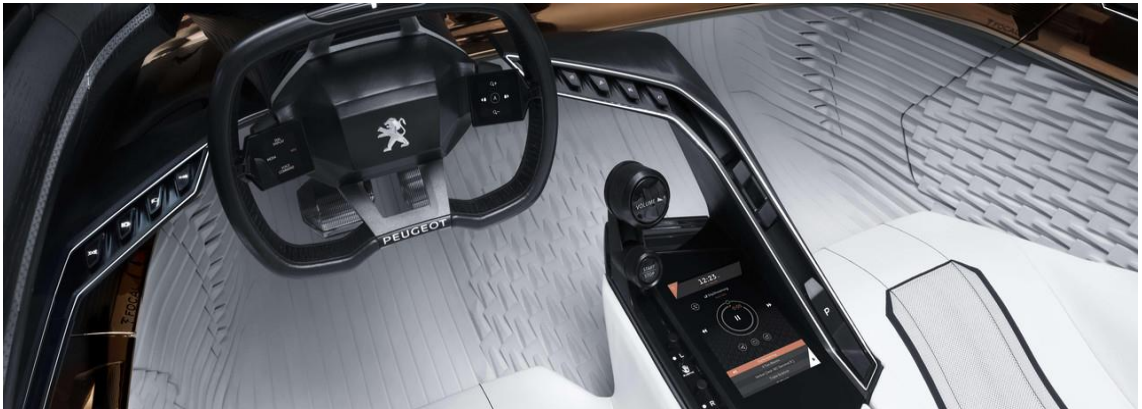
Fig. 3. Peugeot Fractal: sound-absorbing structures, generatively. Source: Peugeot (2015)
