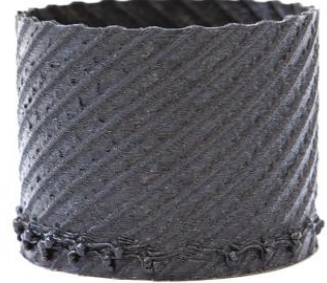
Fig. 3. 24 ribs with 120°, V_{rib} : 400 mm/min, V_{cyl} : 800 mm/min
