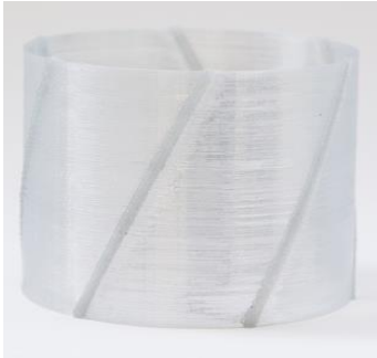
Fig. 1. 6 ribs with 30°, V_{rib} : 400 mm/min, V_{cyl} : 800 mm/min
