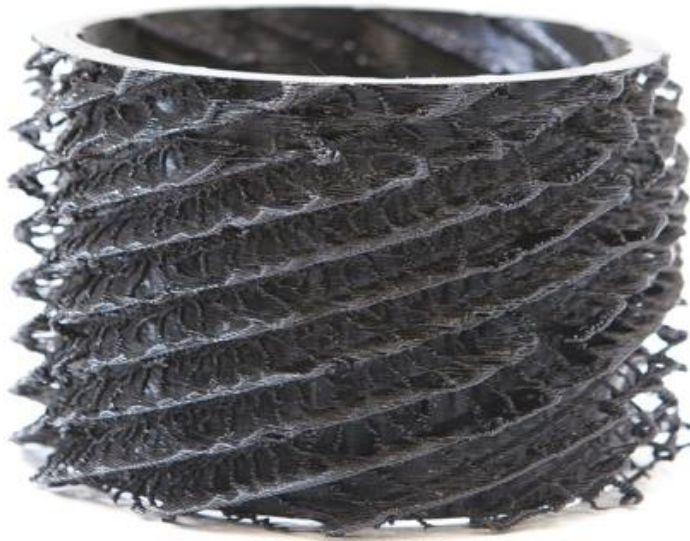
Fig. 7. 18 ribs with 180°, extrusion 5 mm, V_{rib} : 400 mm/min, V_{cyl} : 800 mm/min
